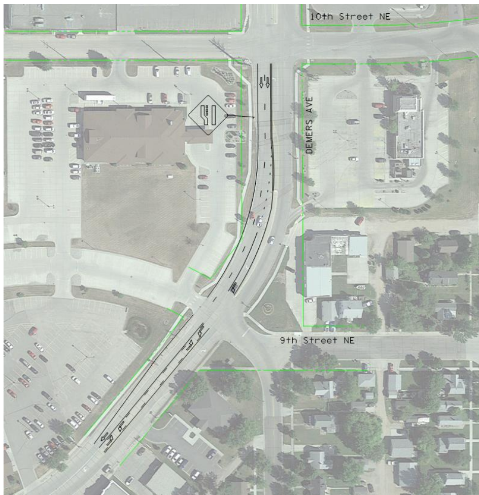
Figure 5-7. Lane Drop and Left Turn Lane Striping Improvement – 10 th Street NE to 9 th Street NE
